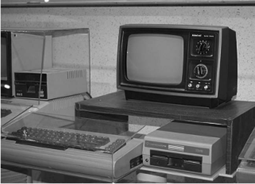
Figure 10.2 The Commodore 64, released in 1982, was a home computer that used the television set as monitor. (Photograph by Dr John Smith, used with permission.)
