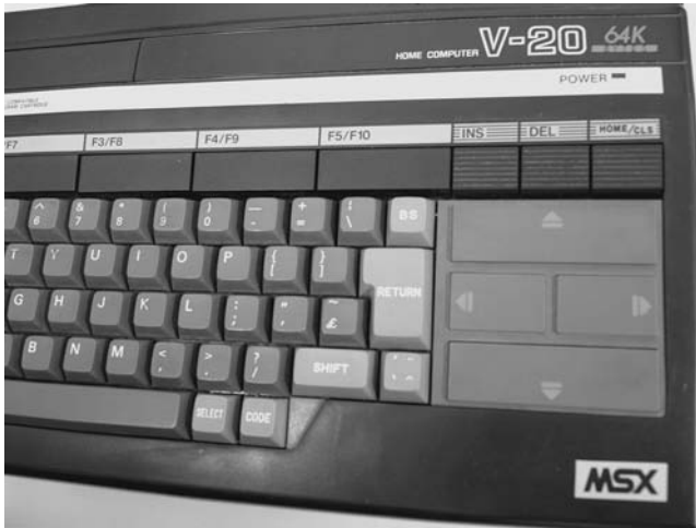
Figure 9.2 The MSX was a hybrid console-computer, popular in Japan in the mid-1980s. Though it looked much like other personal computers of the time, its standardized cartridge format and graphics acceleration made it attractive to game developers. (Photograph by Paolo Tonon. < http://commons.wikimedia.org/wiki/Image:Canon_V-20_MSX_computer.jpg >. Licensed under Creative Commons Attribution ShareAlike 2.0 (CC-BY-SA)).
