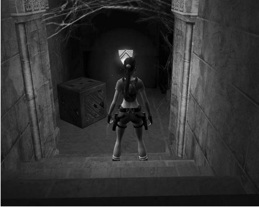
Figure 8.8 Spaces darken as they recede from the player in Lara Croft Tomb Raider: Anniversary (2006) and appear as black beyond a certain distance. This saves render time, since only the areas and objects within a set distance along the z-axis need to be rendered.
