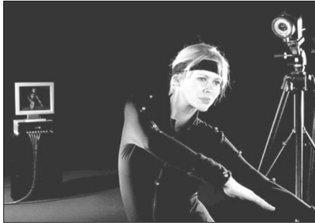
Figure 9.4 A motion capture session. (Note the optical sensors on the black costume.) Image courtesy of Vicon Motion Systems
